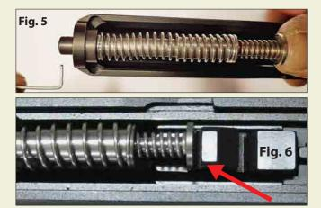
**5.** Assemble the slide on the frame and before loading the magazine, rack the slide several times to ensure that the DPM Rod functions unrestricted.
