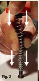
2. Compress at the same time the Spring and the Compressive Disc until you have clear view to the Recoil Rod Assembling Hole (5a) and insert the Safety Pin (Part 5) to block the Washer temporary Fig. 2 a,b
